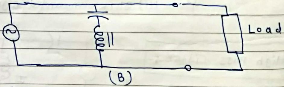
i) Band-elimination, Band rejection, Band-limit, T-notch filter.
