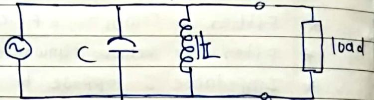
i) Combination of High-pass & low-pass Filter.
