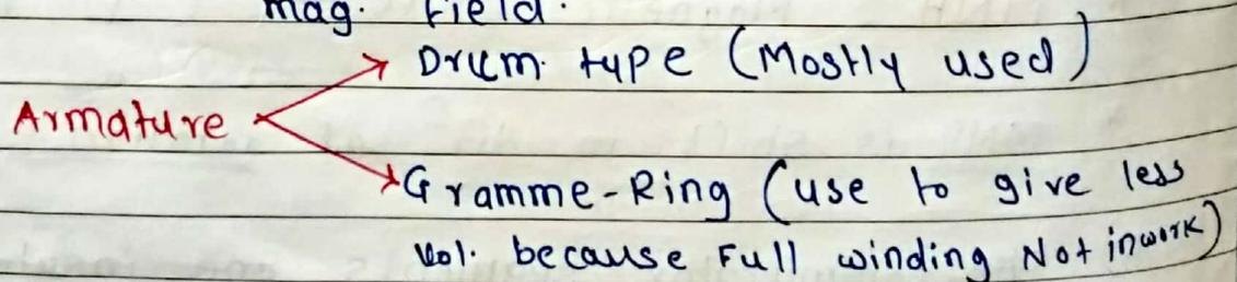
\* Drum type :- Mag. Flux & Vol. induce is greater. Drum type have lap & wave winding method.
